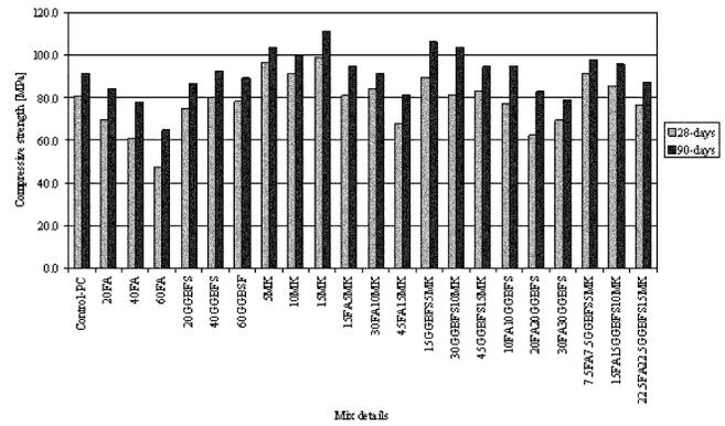
Fig. 3—Variation in compressive strength of SCCs. (Note: 1 MPa = 145.037 psi.)
