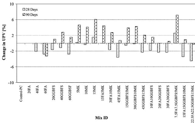
Fig. 6—Normalized UPV values of concretes with respect to control specimen.
