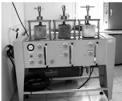
Fig. 1—Testing device for water permeability.
