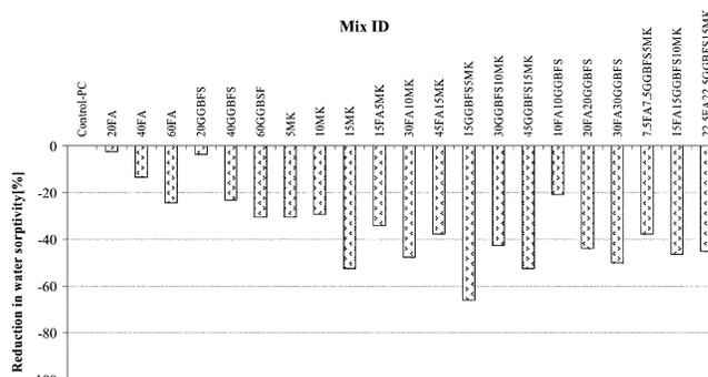
Fig. 9—Normalized water sorptivity of concretes with respect to control specimen.
