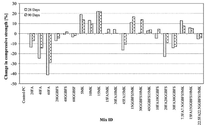
Fig. 4—Normalized compressive strength of concretes with respect to control specimen.
