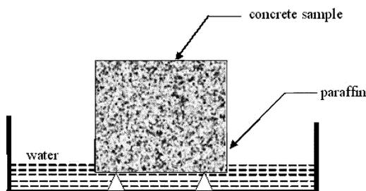
Fig. 2—Sorptivity measurement of SCCs.
