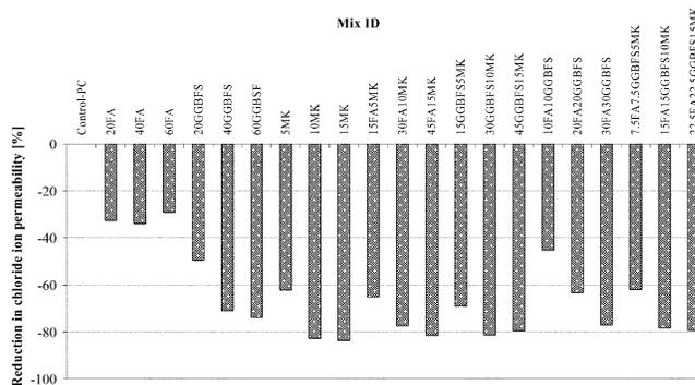
Fig. 7—Normalized chloride ion permeability of concretes with respect to control specimen.
