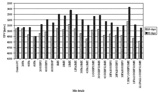
Fig. 5—Variation in UPV of SCCs. (Note: 1 m/s = 3.28 ft/s.)
