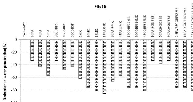
Fig. 8—Normalized water permeability of concretes with respect to control specimen.
