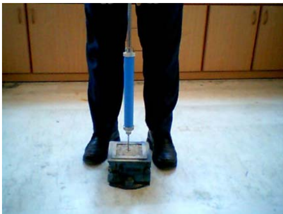
Fig. 3 Measurement of setting times of the mixtures
