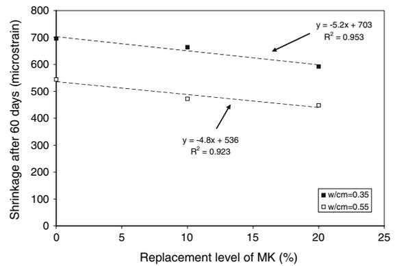
Fig. 6 Relationship between shrinkage after 60 days and replacement level of MK
