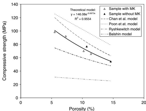
**Fig. 11** Relationship between porosity and compressive strength
