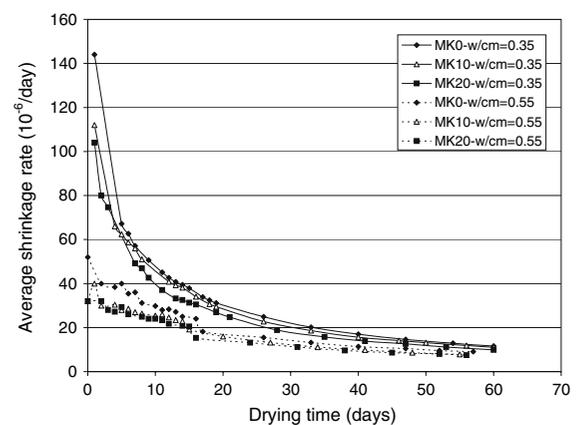
Fig. 7 Average shrinkage rate vs. drying time graphs of plain and MK concretes having w/cm ratios of 0.35 and 0.55
