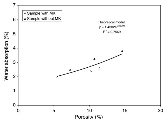
**Fig. 12** Relationship between porosity and water absorption
