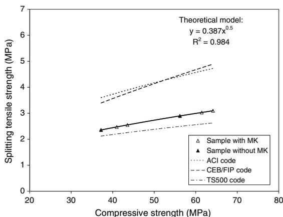
**Fig. 3** Relationship between compressive and splitting tensile strengths
