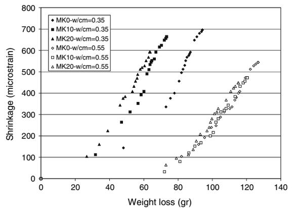
**Fig. 9** Relationship between shrinkage and weight loss
