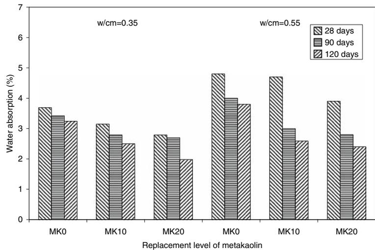
20–29% and 38–45% for the MK concretes, respectively. This reduction in the water absorption with age indicates superior performance of the MK blended cement concretes over the conventional concrete. This may be explained by the pozzolanic activity of MK during the prolonged curing. It is well known that the pozzolanic reactions contribute to the refinement of the binder capillary porosity, with its direct consequences on the improvement of the durability characteristics of the concrete [13].
