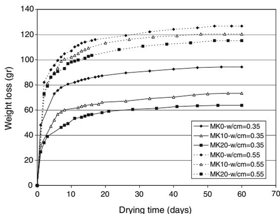
**Fig. 8** Weight loss vs. drying time graphs of plain and MK concretes having w/cm ratios of 0.35 and 0.55
