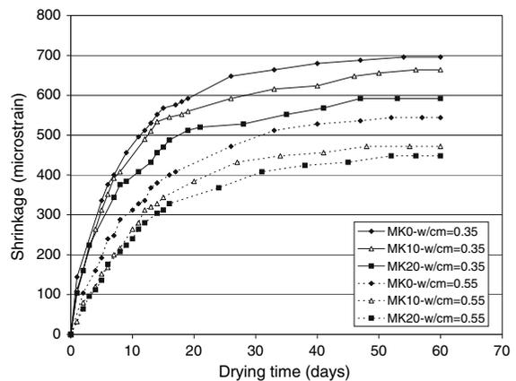
**Fig. 5** Drying shrinkage vs. drying time graphs of plain and MK concretes having w/cm ratios of 0.35 and 0.55
